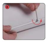
Tighten the top rail screws.
