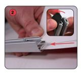
Rotate open the top rail end caps, then squeeze open the grip rail. Slide the graphic squarely into the rail.
